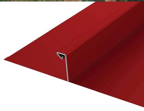
**SPAN-LOCK SL20** is a structural panel that is mechanically seamed during installation. The panel is an integral interlocking system by design which installs in one direction from a given starting point. The Span-Lock is a very flexible panel that works well with a wide range of building designs.
