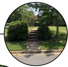
In order to preserve the existing 8" diameter Ginkgo tree, and to maintain the existing lead walk from #621 Blackstone Terrace the sidewalk would be built against the curb (without a utility strip). The Arborist has noted that the Ginkgo tree is in "Excellent" condition.
