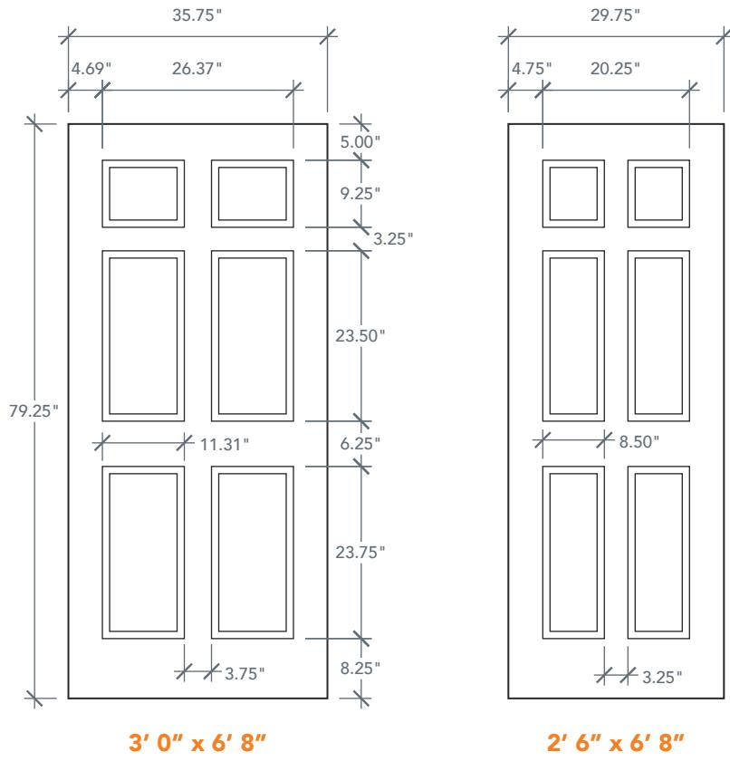
NOTE: BY REQUEST, DOOR HEIGHT COMES IN VARYING DIMENSIONS TO A MINIMUM OF 79". EXCESS WILL BE TAKEN FROM BOTTOM RAIL. ALL OTHER DIMENSIONS WILL REMAIN THE SAME.
