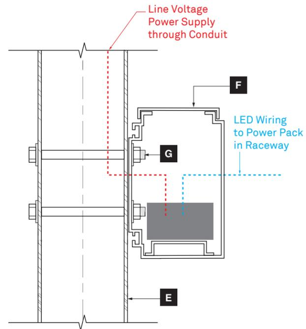
**B** Detail - Raceway Attachment
