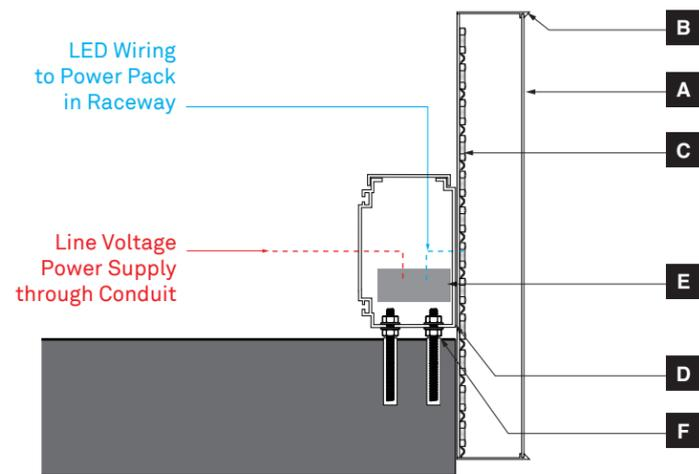
**A** Section - Storefront Sign - Raceway Mounted - Sign Band
