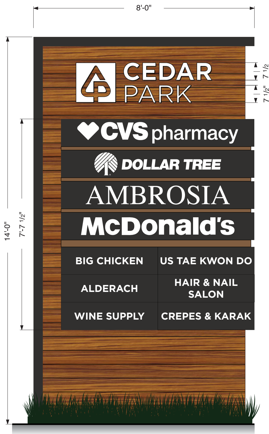
A Left Face - Elevation - Multi-Tenant Pylon 1/2" = 1'-0"
