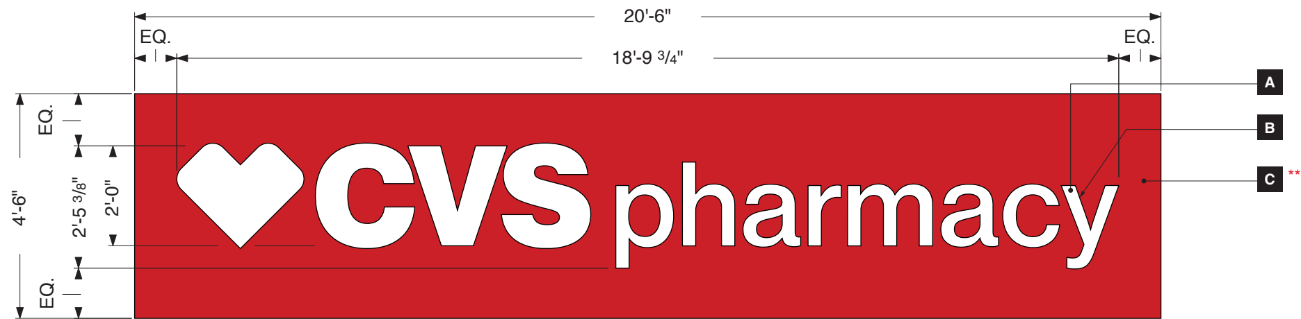
B Detail Elevation - Junior Anchor Tenant Sign 3/8" = 1'-0"
