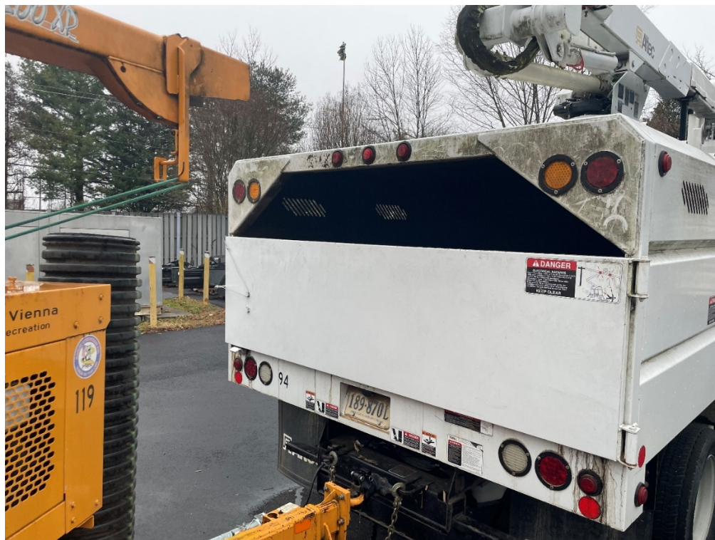
Figure 3 - Note the height difference of the chipper chute and the atypical narrow opening of the chip box.
