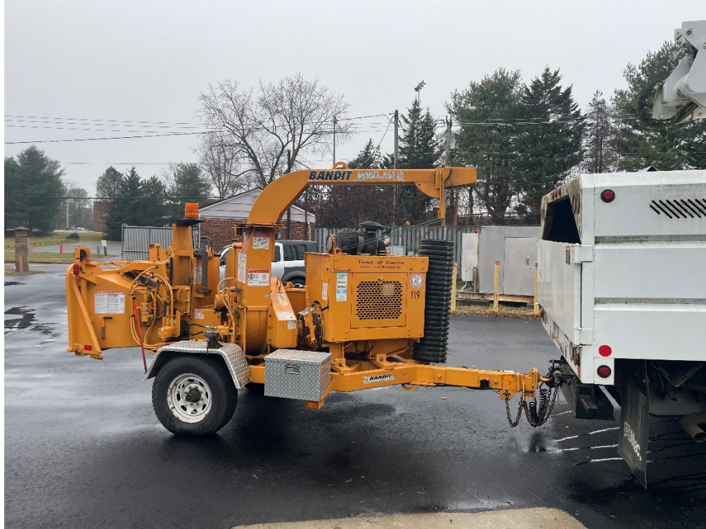
Figure 2- Chipper is adequate however note the height incompatibility from the chipper chute to the chip box.
