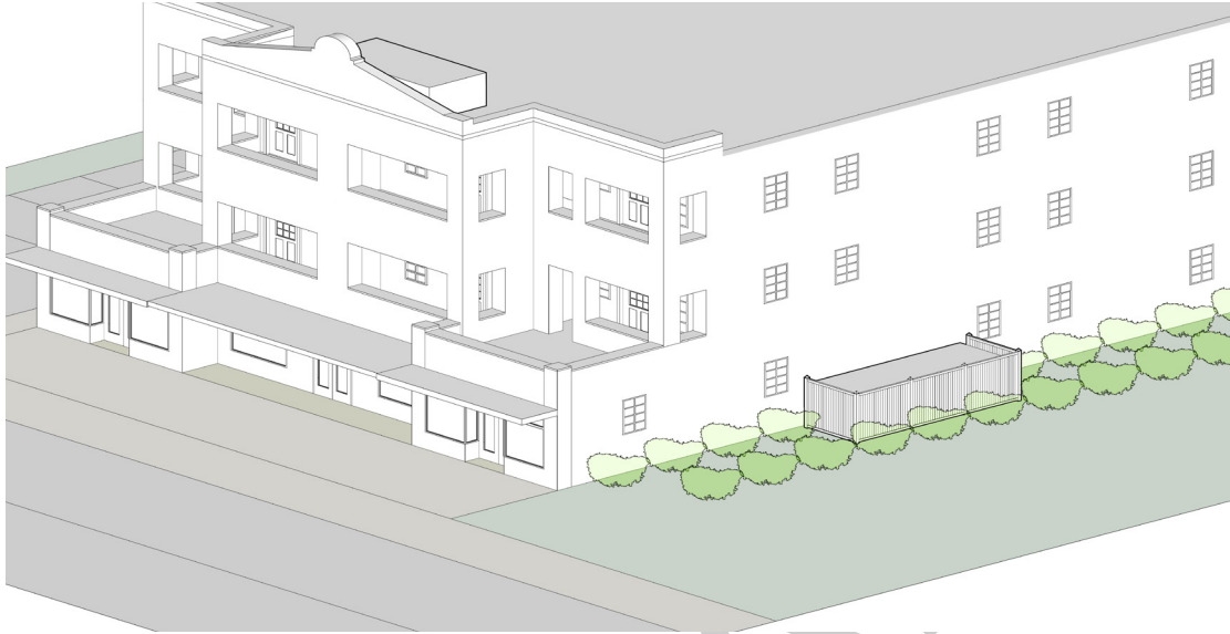
FIGURE 5.A. Illustration of screening around ground-level mechanical equipment.
