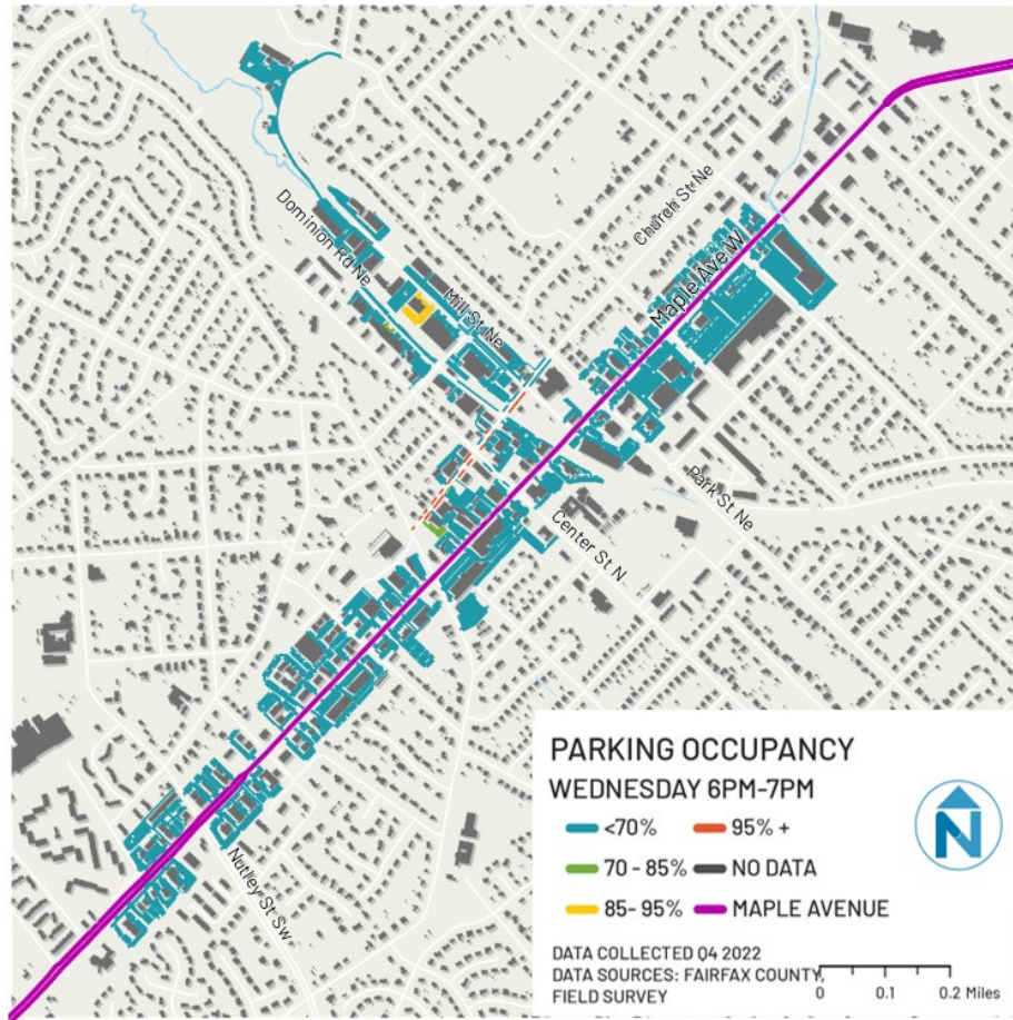
Figure 5: Parking Utilization – Wednesday 6pm
