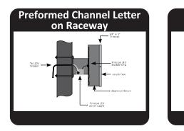
Specs: Two sets Preformed channel letters w/ polycarb faces and LED's - raceway mounted Face: White polycarbonate w/ Light Blue, Navy, Red & White vinyl applied as per artwork. Trim: 1" Black Return: 4 pre-finished Black / Interiors White. Illumination: Principal QwikMod White PLQM2-TW150-P. 7100K, 118lm/w, 94.1 lm/mod. Power Supplies: Principal P-OH060-12-EC 90-305VAC - rwy.
