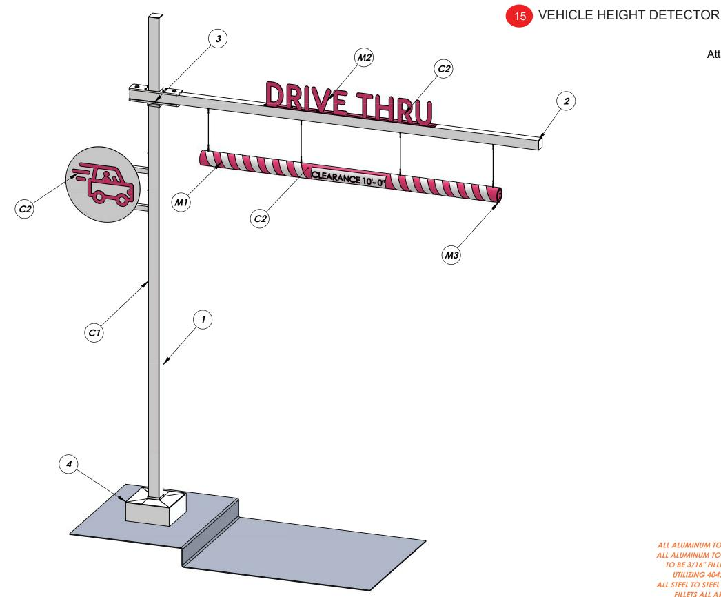
ALL ALUMINUM TO BE 6061-T6 U.N.O. ALL ALUMINUM TO ALUMINUM WELDS TO BE 3/16" FILLETS ALL AROUND UTILIZING 4043 FILLER U.N.O. ALL STEEL TO STEEL WELDS TO BE 3/16" FILLETS ALL AROUND U.N.O.
