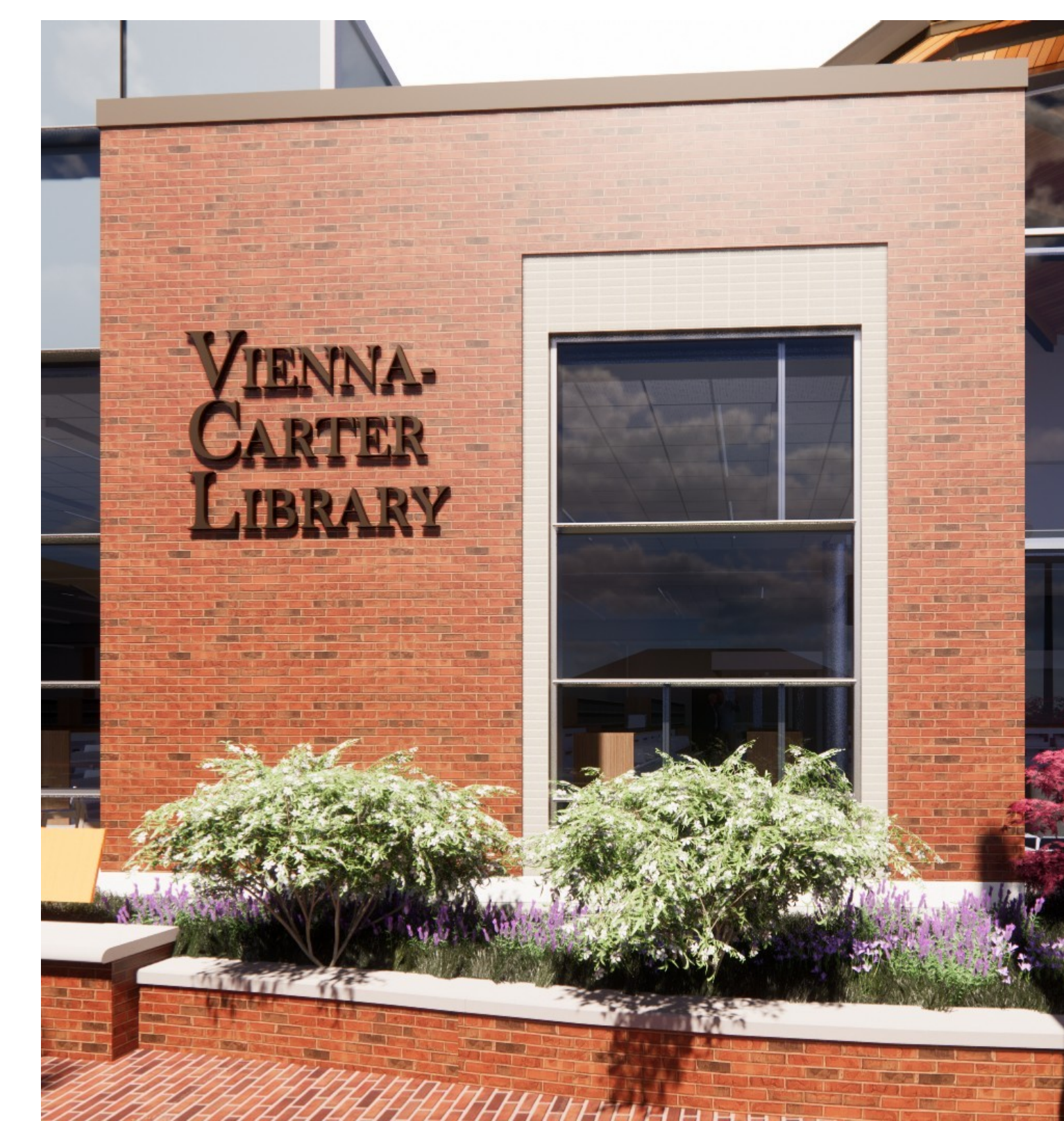
5 CUT LETTER BUILDING SIGN SIGNS SCALE: 3/8" = 1'-0" 1/2" THICK ALUMINUM CUTOUT LETTERS, CONCEALED STUD MOUNTING TO FACE BRICK
