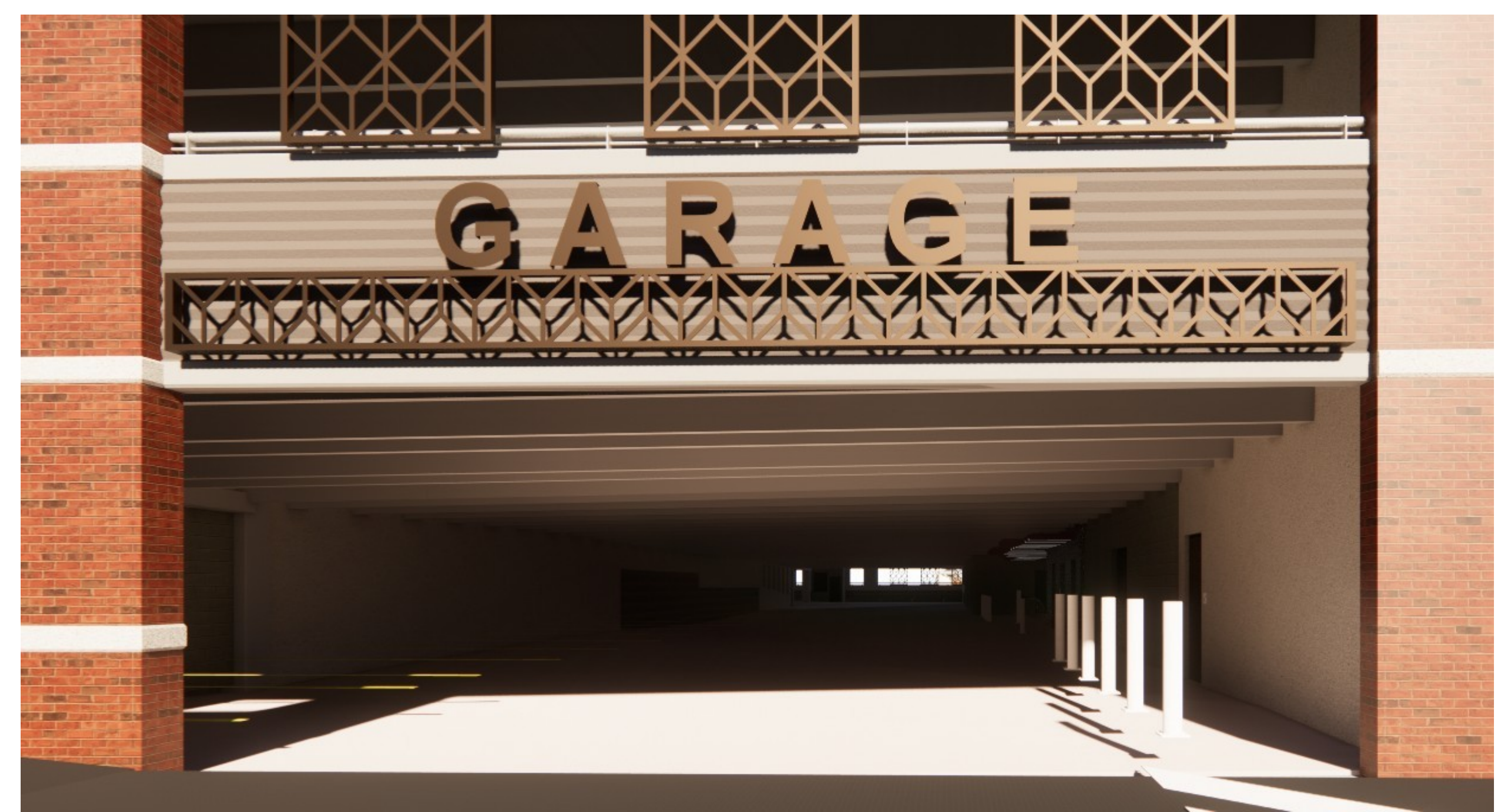
6 UPRIGHT CHANNEL LETTER GARAGE SIGN SIGNS SCALE: 3/8" = 1'-0" ALUMINUM CHANNEL LETTERS W/ 2" RETURN EDGES MOUNTED ON ALUMINUM CUTOUT PANEL STUD ATTACHED TO GARAGE PRECAST CONCRETE SPANDREL PANEL
