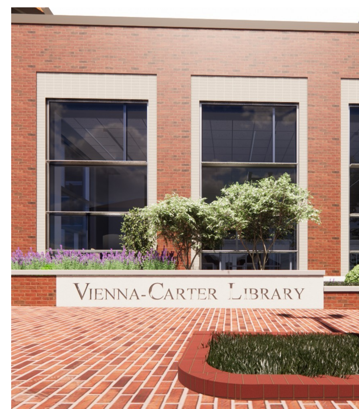
4 CAST STONE BUILDING SIGN SIGNS SCALE: 3/8" = 1'-0" CAST STONE PANEL(S) WITH ENGRAVED LETTERS
