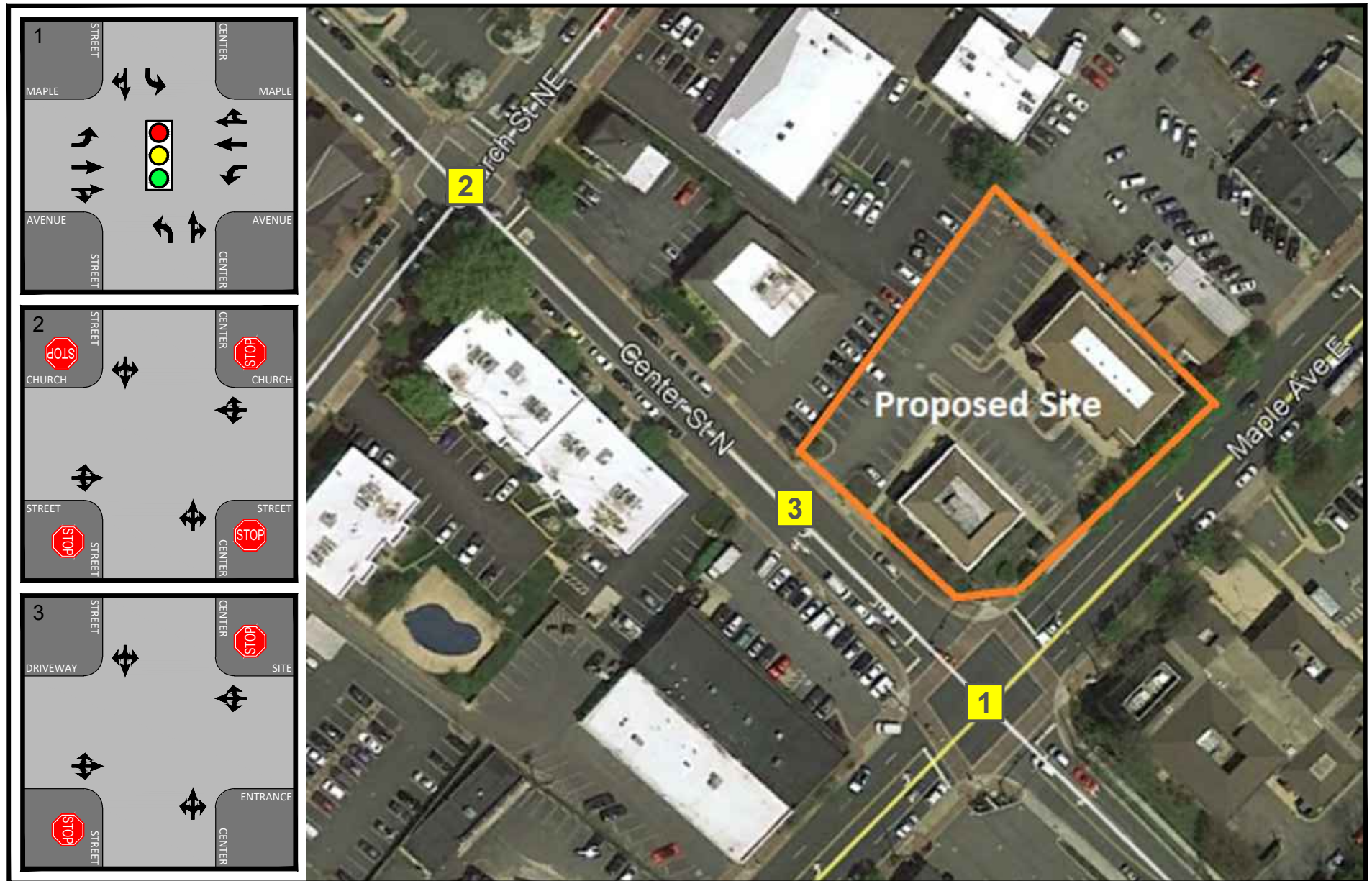
Figure 5-2 Future Lane Use and Traffic Controls
