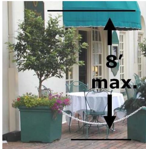
Planters may be used in addition to or in place of other barrier designs. In addition, planters may be used in situations where no barrier is required (for example, where the outdoor dining area does not extend more than three feet into the sidewalk) in order to provide added visual interest and create a more attractive and welcoming atmosphere. Planters must be easily moved by one person and shall not create a continuous barrier that cause an obstruction to Fire Department access.
