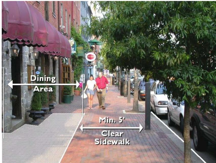
*Outdoor dining areas must leave at least five feet of unobstructed pedestrian space, including between the base of barriers. On sidewalks the five-foot passage way must form a continuous linear path in front of the business as illustrated in the example.*
