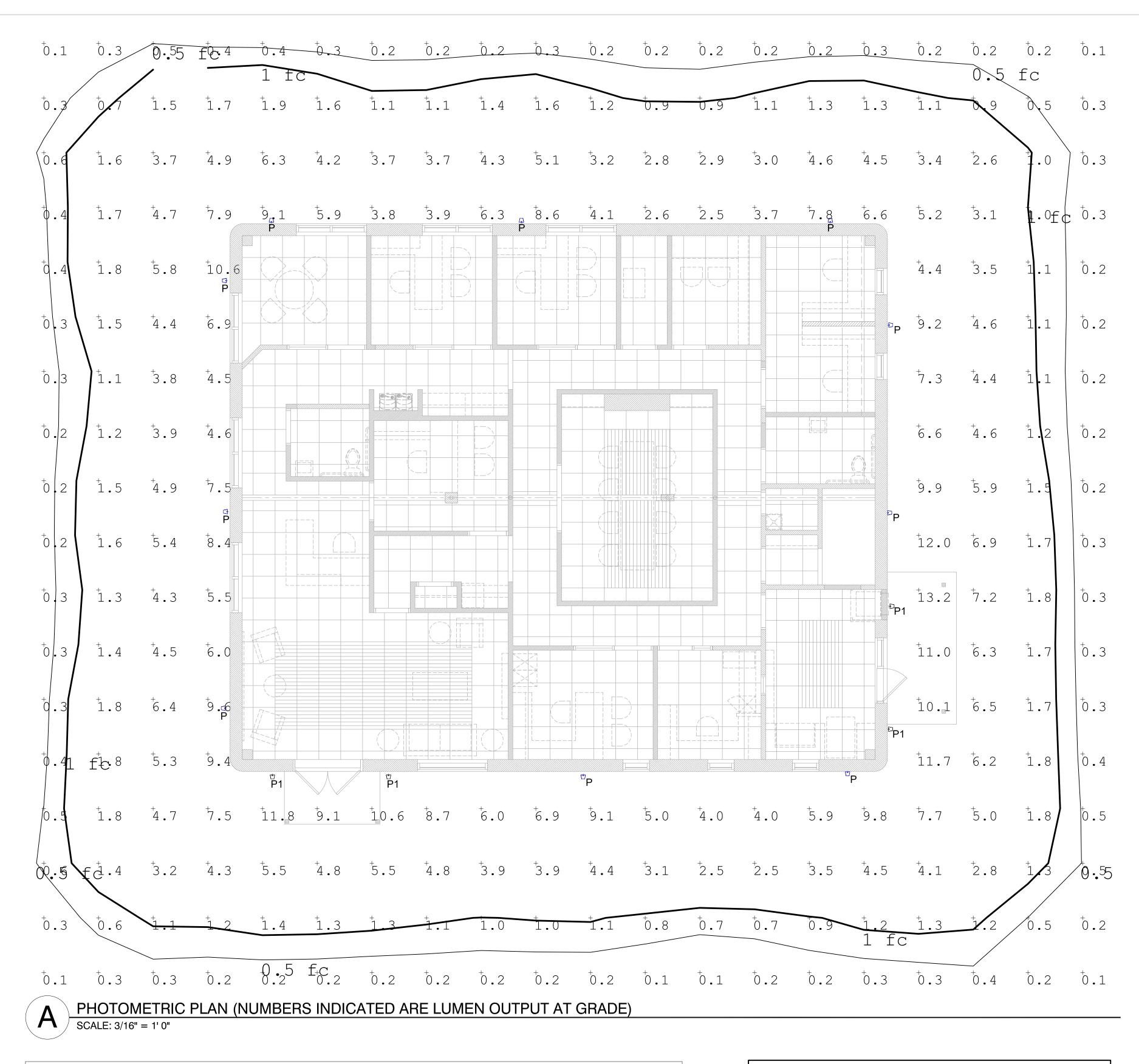
Luminaire Schedule Qty Arrangement LLF Description Arr. Watts 0.850 | Lithonia Lighting WSQ LED P1 SR3 40K MVOLT DDBXD 19.56 Single 0.850 Lithonia Lighting WSQ LED P1 SR3 40K MVOLT E20WC DDBXD 19.56 Single
