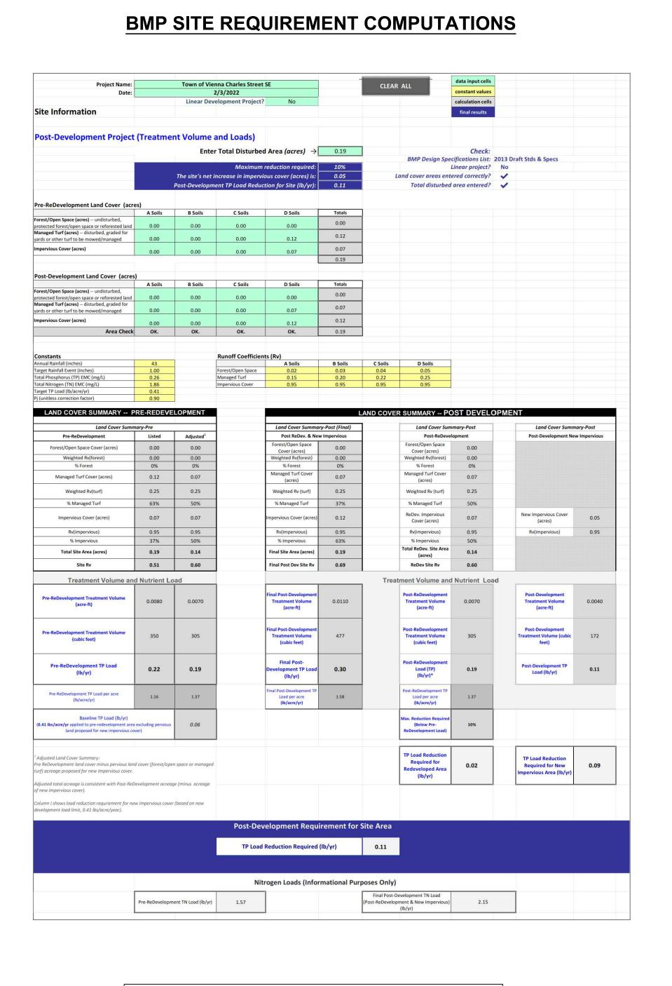
NOTE: THE COMPUTATIONS SHOWN ON THIS SHEET WERE DETERMINED USING VERSION 3.0 OF THE VIRGINIA RUNOFF REDUCTION METHOD (VRRM) RE-DEVELOPMENT COMPLIANCE SPREADSHEET RELEASED MAY, 2016.
