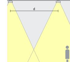
Linear lighting For uniform lighting with luminaires arranged in a line, the spacing (d) between two Light-scan surface-mounted downlights should be the height (h) of the luminaire above the working plane.
