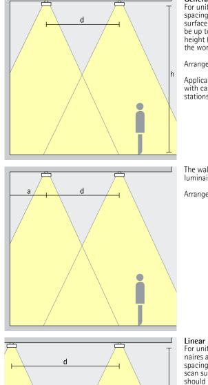
**General lighting** For uniform ambient lighting, the spacing (d) between two Lightscan surface-mounted downlights may be up to approximately half the height (h) of the luminaire above the working plane.
