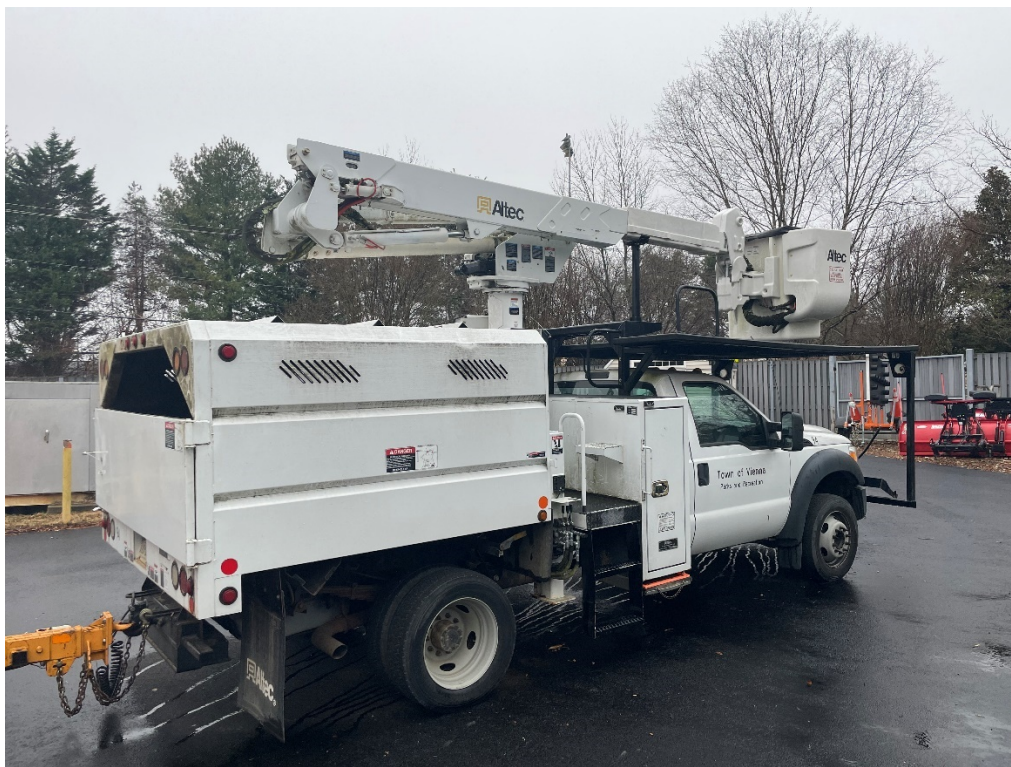
Figure 1- Aerial lift with short boom, small chip box and narrow opening for wood chips.
