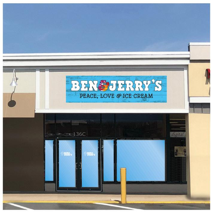
Set of LED illuminated (100 lumens or less) raceway channel letters for "Ben & Jerry's" with blue background made from aluminum composite material blue vinyl applied, black/grey line overlay mounted on raceway, raceway mounted on sign band.
