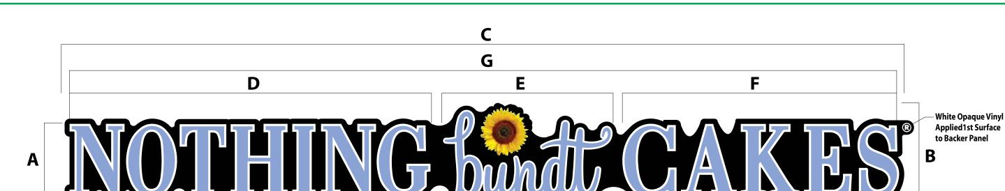
Qty: 1 - Front Elevation Illuminated Raceway Mounted Blue Channel Letters Mounted on Black Backer Panel (Brightness - 30 Lumens)
