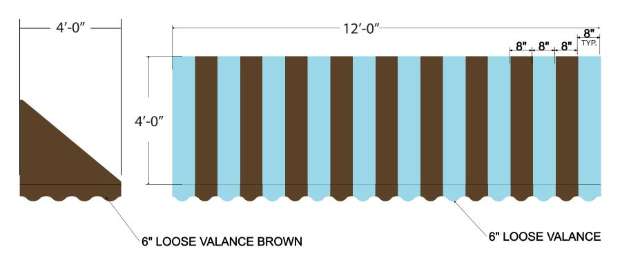
**AWNING:** FABRIC / CLOSED ENDS **AWNING TYPE:** SHED STYLE W/ 6" LOOSE VALANCE **MANUF.**: "SUNBRELLA" 6021 TRUE BROWN W/ 3M 3630-317 EVENING BLUE LAMINATED TO WHT. OPAQUE FINISH TBD **FRAMING:** MOUNT TO BULKHEAD OVER GLAZING **MOUNTING:**
