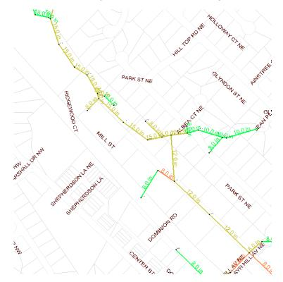
**Table 7** below shows the proposed pipe size improvements for the NW sewershed to handle the wet weather flows in both existing conditions and buildout scenarios.
