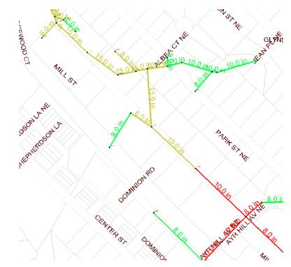
Pipe Improvements Alt. 2 – Mill Street - North of Ayr Hill Av (10-inch to 12-inch) Existing Conditions Wet Weather.
