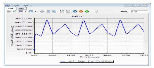
It is to be noted that the model "peaks" and "valleys" closely match the flow values recorded at the sewer meter locations and the model is calibrated for a typical "dry-weather" scenario within the scope of the modeling assumptions. Additional calibration may be required if the Town plans to conduct flow monitoring within each sewershed or specific area of interest.
