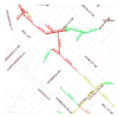
The figure below shows the impact of the pipeline improvements for the Maple Street Commercial Development wet weather scenario. This scenario assumes the pipe upsizing proposed in both alternative 1 and alternative 2.
