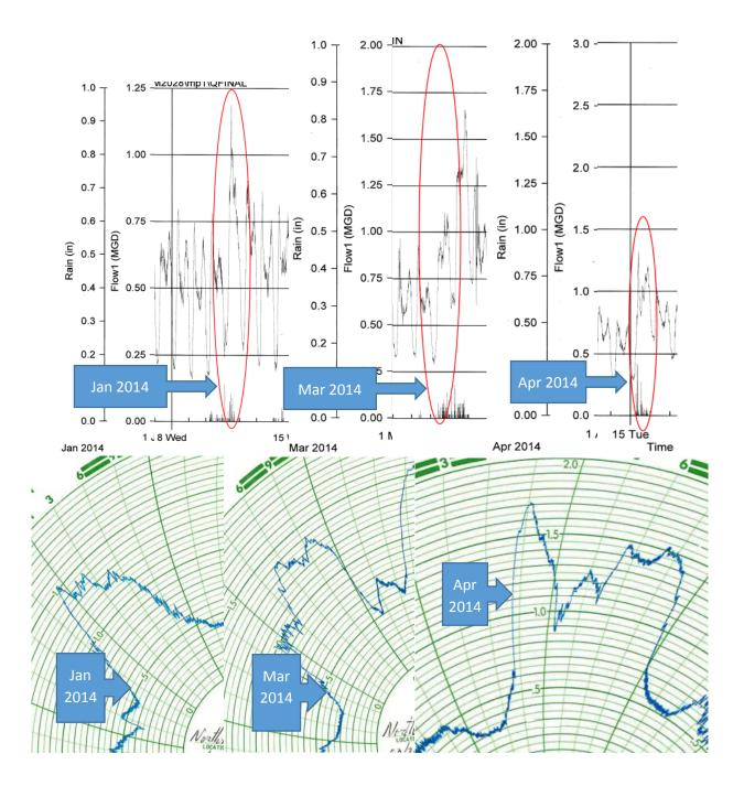
A wet weather scenario was simulated for all sewersheds to identify capacity constraints within the existing sewer network. This was accomplished by adding the additional flow due to I&I to each flow node. This additional flow was derived by utilizing a multiplication factor observed at the flow meter at that sewershed during a routine wet weather event. The "wet weather" meter data is included in **Appendix B**.
