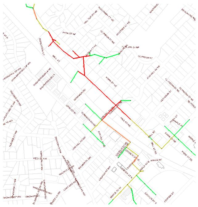
This existing condition wet weather scenario indicates that the existing 10-inch and 12-inch lines along the Mill Street corridor are deficient. This confirms the issue that Town has had with the sanitary sewer along Mill Street. SSO and manhole surcharging has been recorded at several locations along Mill St. based on the current modeling assumptions.
