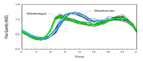
The diurnal pattern for each sewershed was developed by evaluating the data from each flow meter at the four discharge locations and selection of a common "dry-weather" day. The "peaks" and "valleys" in the recorded data were compared to the recorded average flow to create the unitless diurnal pattern. The peak flows were observed at 9:00 AM in the morning.
