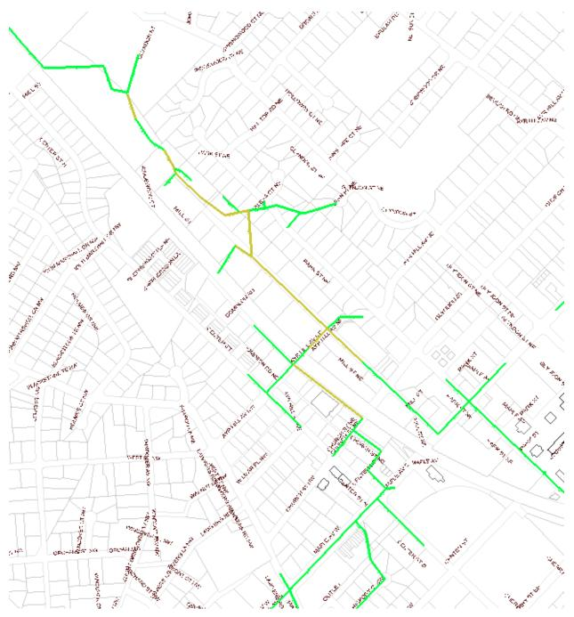
The figure below shows a color coded graphic of the sewer network for the Maple Ave Development and dry weather scenario. The yellow line type indicates that the sewer flow has exceeded 50% the available pipe capacity.
