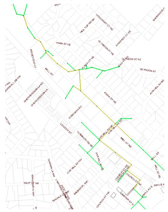
The figure below shows a color coded graphic of the sewer network in an existing condition wet weather scenario. The red line type indicates that sewer flow has exceeded 99% the available pipe capacity, the orange indicates 80% exceedance and the yellow indicates 50% exceedance.
