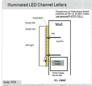
t This sign is intended to be installed in accordance with the requirements of Article 600 of the National Electrical Code and/or other applicable local codes, his includes proper grounding and bonding of the sign.
