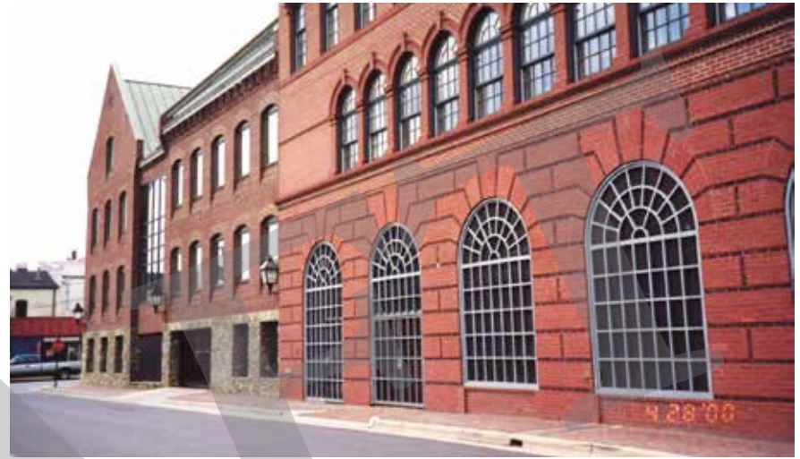
The parking level of the structure should be detailed to look like the rest of the building while still screening the parked cars.
