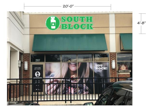
SIGN INSTALLED OVER STOREFRONT CENTERED LEFT TO RIGHT AND 2" HIGH OF CENTER TOP TO BOTTOM Date : 01/29/20
