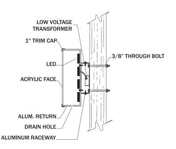
(1) SET OF INDIVIDUALLY ILLUMINATED CHANNEL LETTERS INSTALLED ON 1st LEVEL OF STOREFRONT
